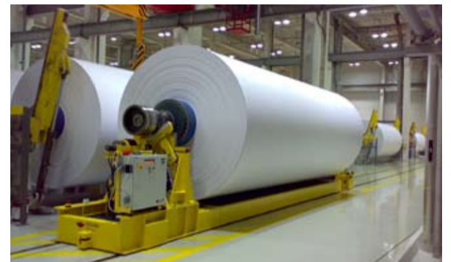
Solving AGV Movers handle 4000 kg cardboard rolls from storage to further processing in Forshaga, Sweden.
