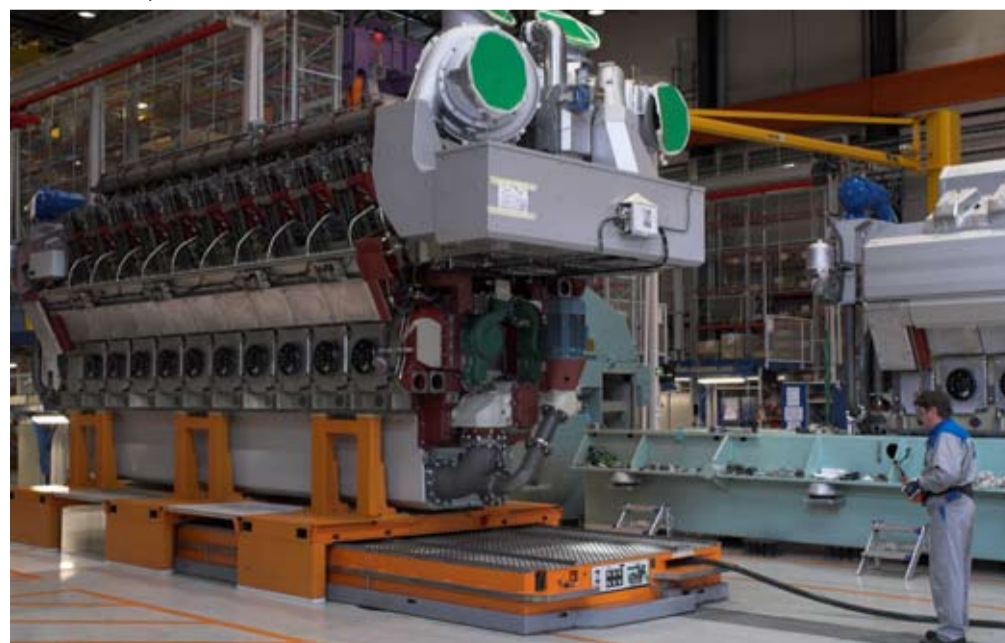
A 100-tonne diesel engine is floated smoothly on air bearings through production.
