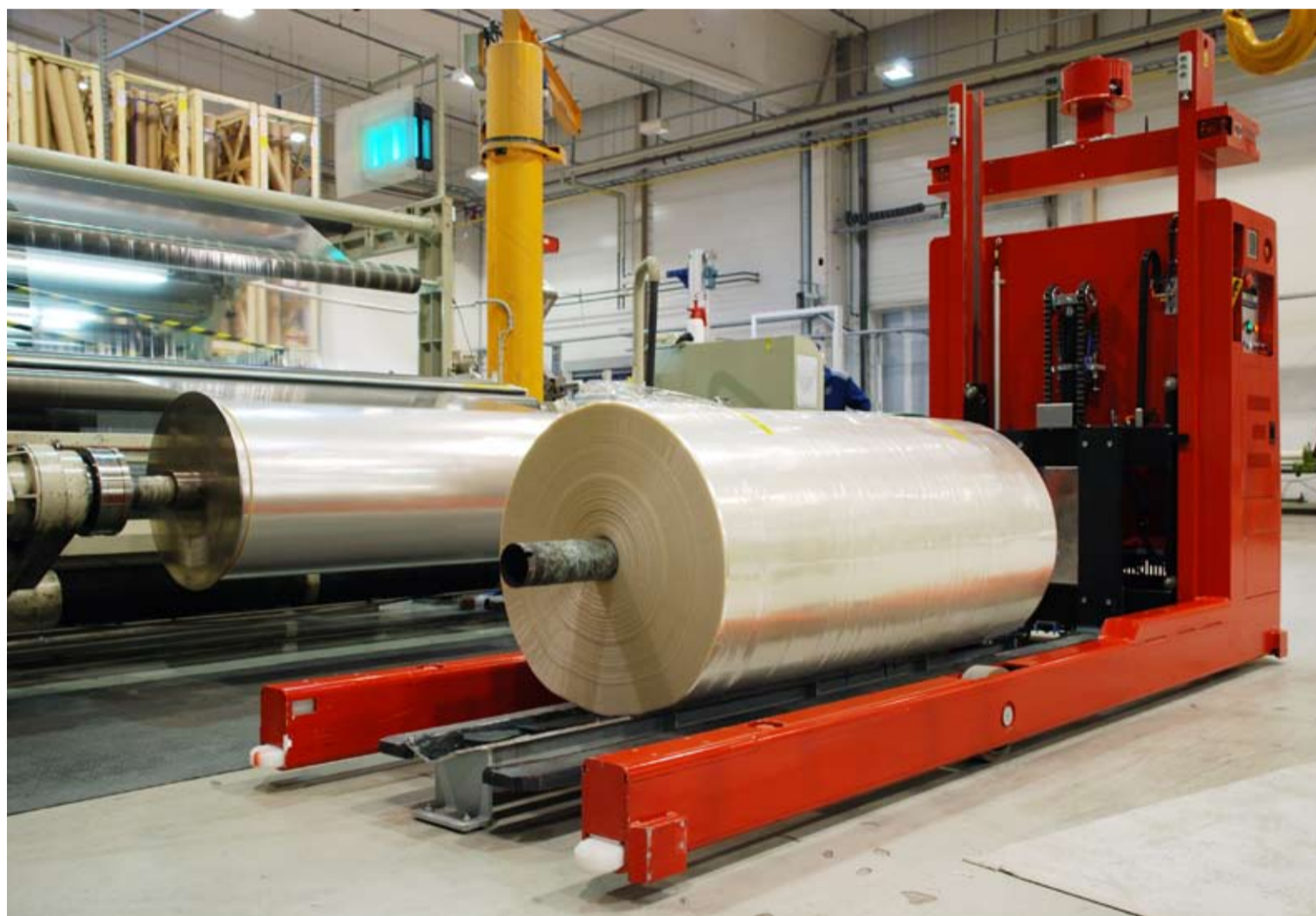
Laser guided Solving AGV Movers handle plastic rolls from production to storage. Page 3.
