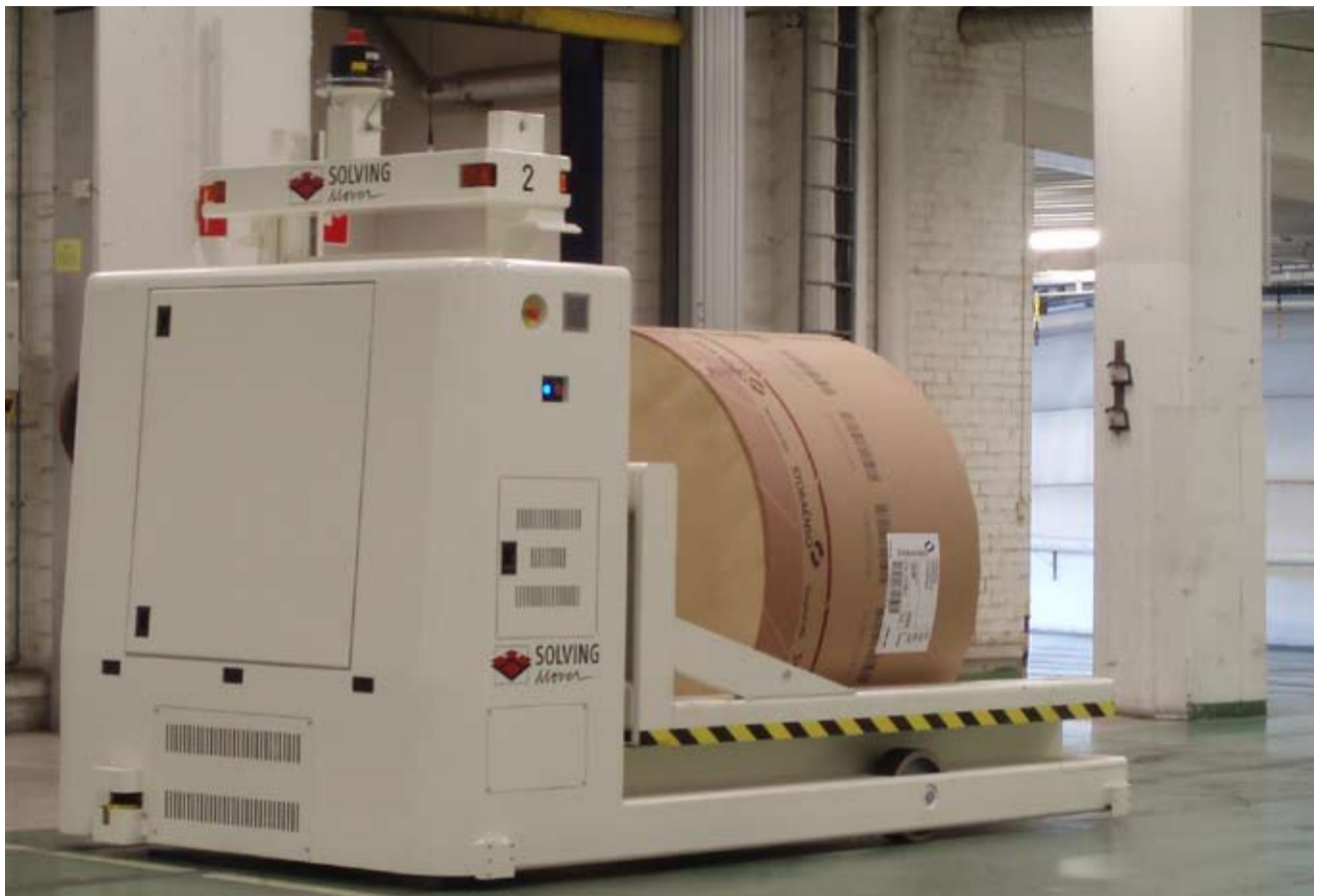
Solving AGV Movers handle 4000 kg cardboard rolls from storage to further processing in Forshaga, Sweden.
